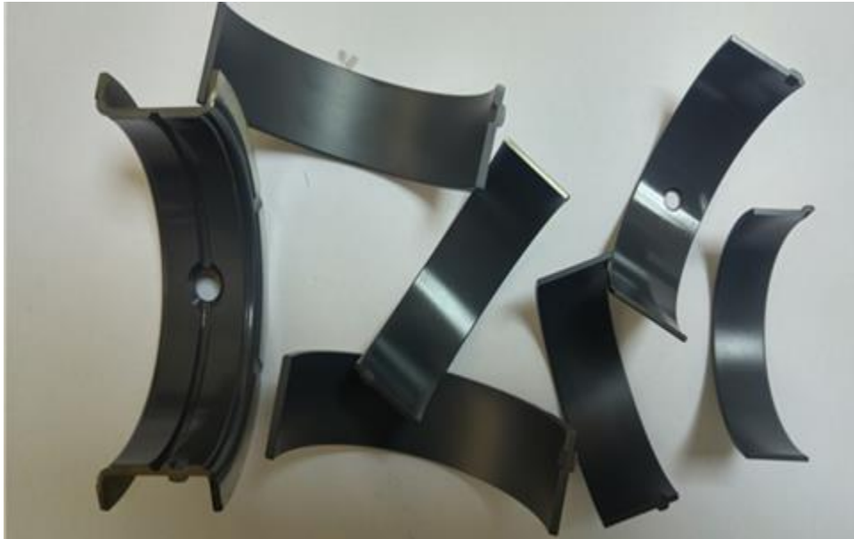
Fig.3 Polymer coated King race bearings
